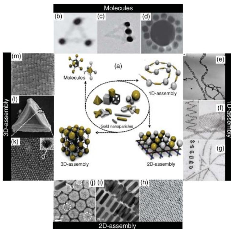
**Fig. 4.** (a) Schematics of various assemblies from constituting nanoparticles (adapted from Ref. 100; image has been modified from the original figure). **b–d** (adapted from Ref. 100), **e–g** (adapted from Refs. 100 and 102), **h–j** (adapted from Refs. 100,90, and 103), and **k–m** (adapted from Refs. 113 and 114) are molecular, one-, two-, and three-dimensional assemblies, respectively, made of various GNPs. **k** is an expanded TEM image of a portion of superlattice shown in **l**.
