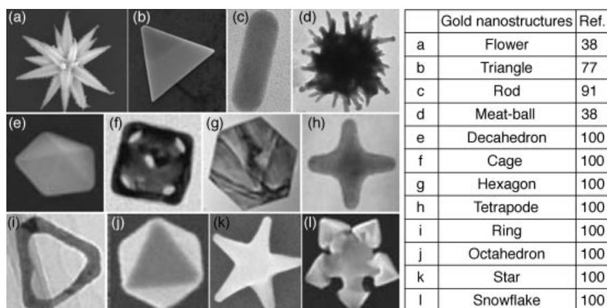
**Fig. 3.** Microscopic images of various anisotropic GNPs. References from which the images are taken are indicated in the table. The particles occur in the size range of 30 nm to 10  $\mu$ m.
