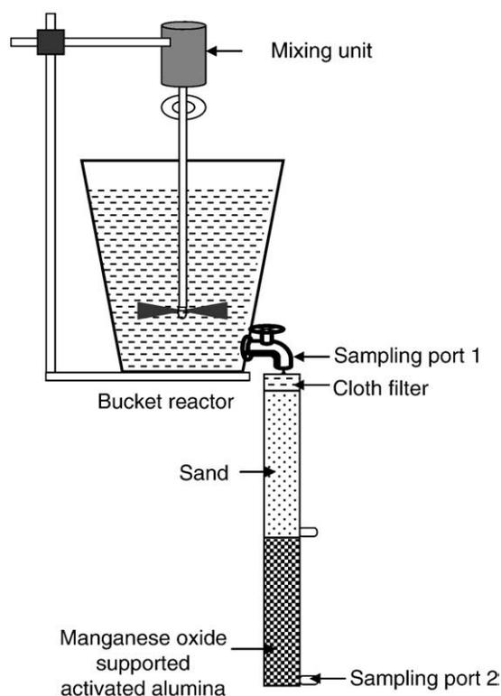
Fig. 1. Schematic of a household defluoridation unit (HDU).
