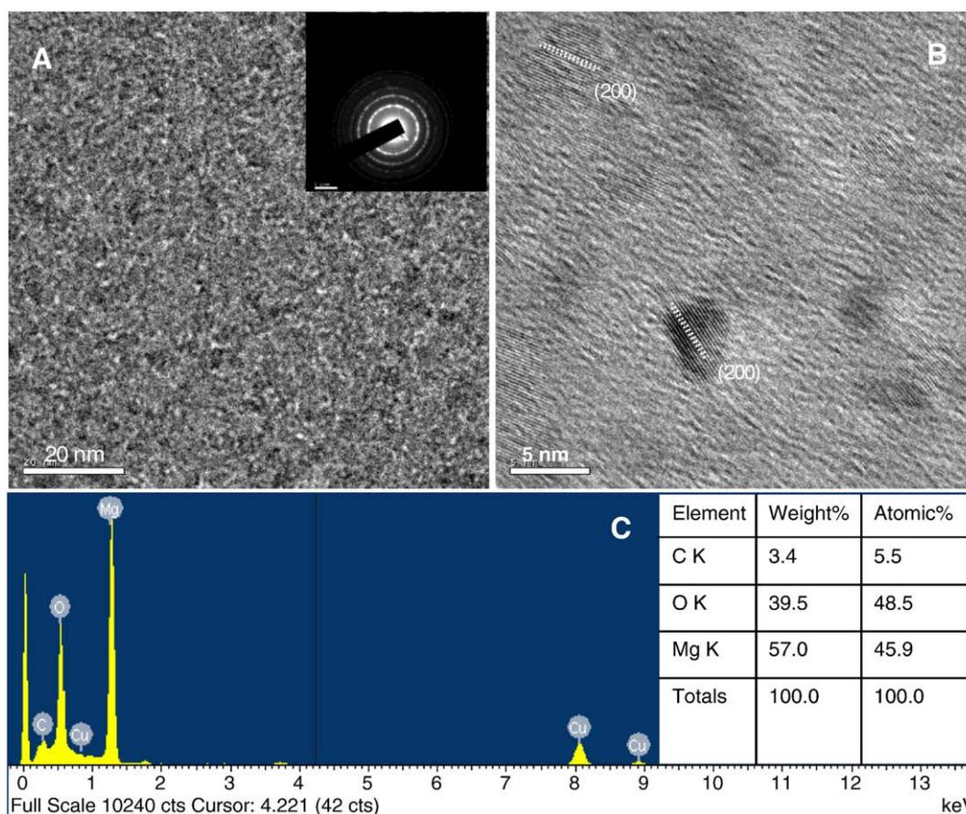
**Fig. 4.** TEM images of (A) as-synthesized NM (inset: SAED pattern) (B) a particle from (A) is expanded (C) EDX spectrum of as-synthesized NM (inset: elemental composition of as-synthesized NM). Note that the grid used was carbon coated copper.
