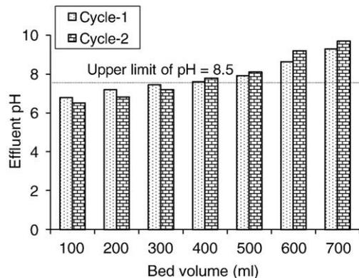
Fig. 11. Hydroxyl ion uptake capacity of manganese oxide-supported-activated alumina.
