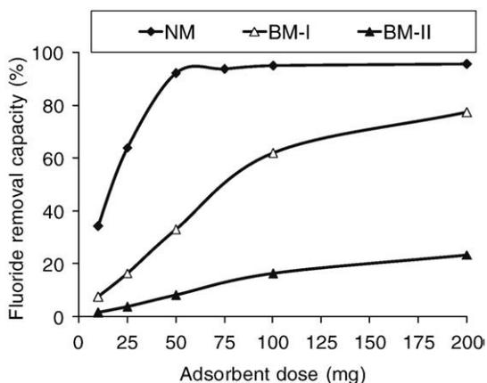
Fig. 6. Effect of adsorbent dose on fluoride removal (initial fluoride conc. = 10 mg l<sup>-1</sup>). Legends—NM: as-synthesized nano MgO; BM-I: MgO light (Thomas backer limited, Mumbai, India); BM-II: bulk MgO (Commercial grade).
