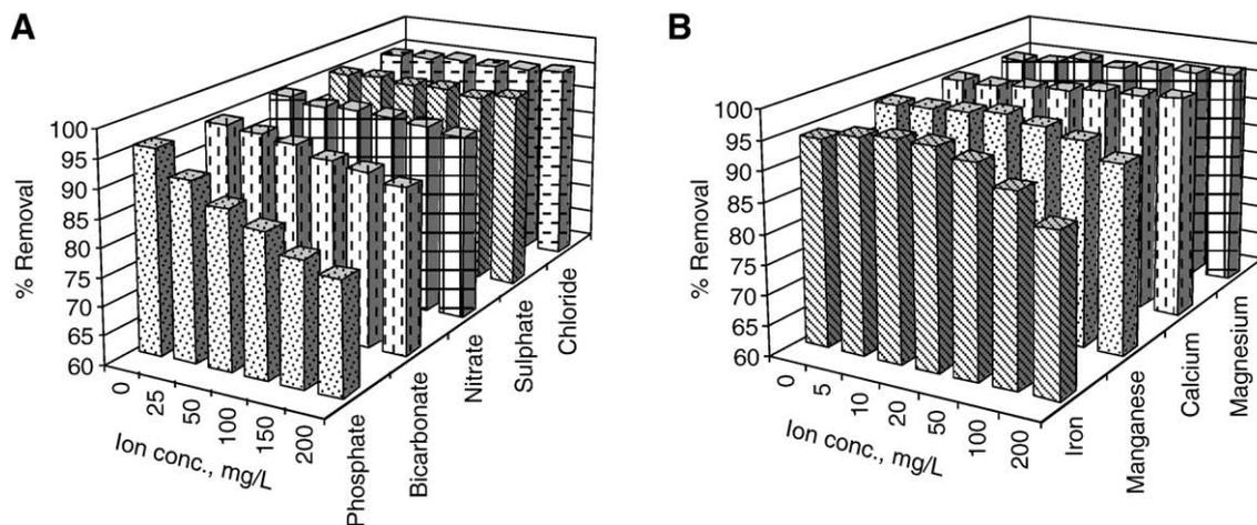
Fig. 10. Effect of various background (A) anions and (B) cations on the fluoride removal capacity by NM (initial fluoride concentration = 10.0 mg l<sup>-1</sup>, pH 7 ± 0.1).
