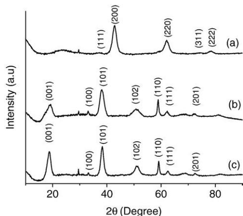
Fig. 2. XRD spectra of (a) as made NM (b) Hydrated NM (c) NM after reaction with 50 mg l<sup>-1</sup> fluoride. The traces are shifted vertically for clarity.
