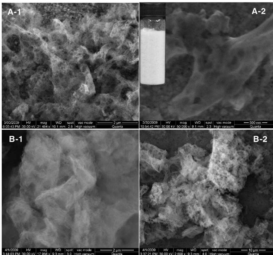
Fig. 3. SEM micrographs of (A-1, A-2) as-synthesized NM and (B-1, B-2) NM after reaction with fluoride. Inset of A-2 is a photograph of the as-synthesized NM.
