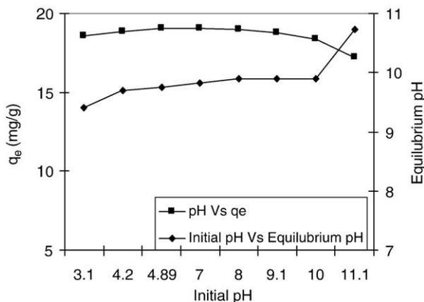
Fig. 9. Effect of pH on fluoride adsorption by NM (initial fluoride conc. = 10 mg l<sup>-1</sup>, temperature = 30 ± 2 °C).
