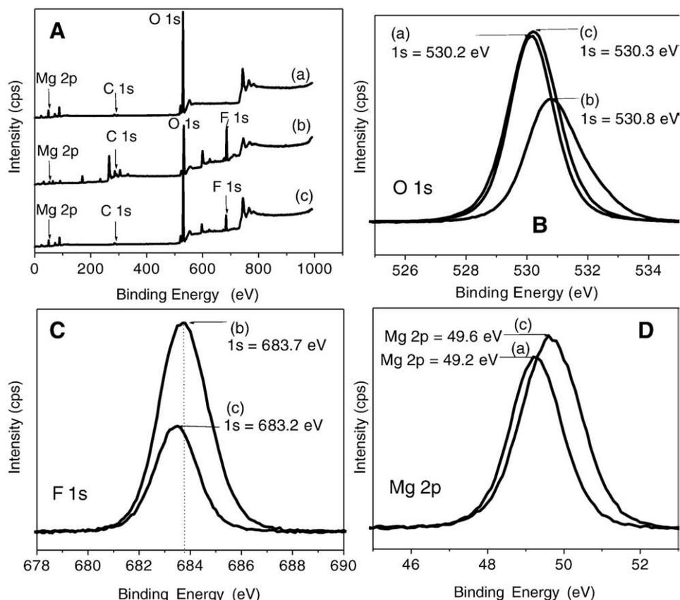
Fig. 5. XPS spectra of (a) hydrated NM, (b) MgF<sub>2</sub> (supplier: Leo Chem, Bangalore, India and (c) NM after reaction with 50 mg l<sup>-1</sup> of fluoride. Various regions (O1s, F 1s and Mg 2p) are expanded.
