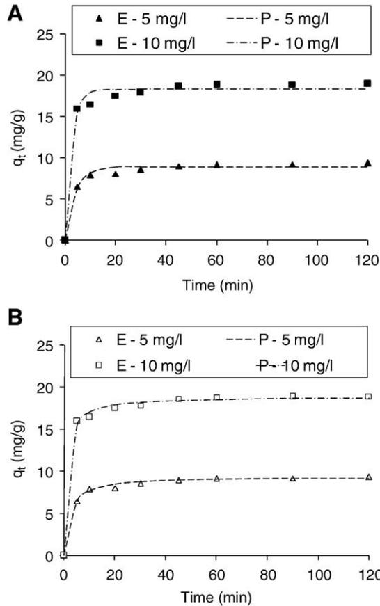
Fig. 7. Comparison of (A) pseudo-first-order and (B) pseudo-second-order kinetic plots with experimental data for adsorption of fluoride by NM (E–experimental; P–predicted).
