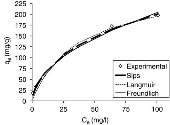
Fig. 8. Comparison of various isotherm models for fluoride adsorption onto NM (temperature –  $30 \pm 2^\circ\text{C}$ ).
