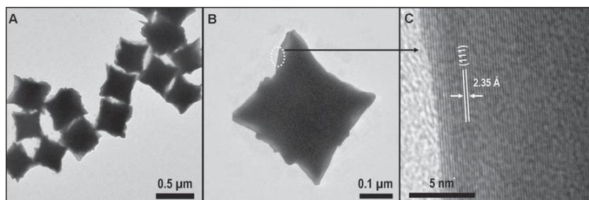
**Fig. 4.** TEM images of the cube-like mesostructures synthesized by using 0.6 M 1,2-PDA during the seed preparation. (A) Large area image; (B) single cube-like mesoparticle and (C) lattice resolved image.
