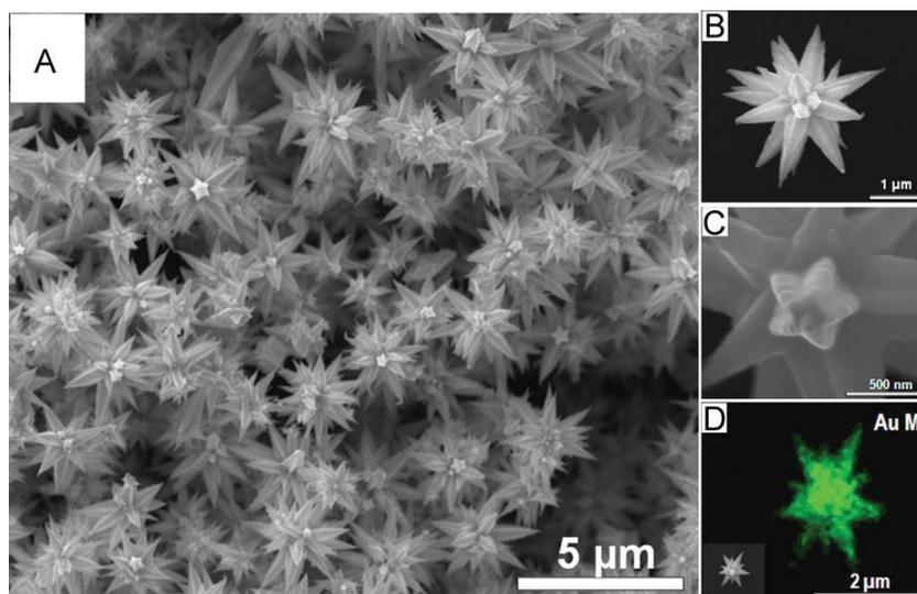
**Fig. 1.** (A) A large area SEM image of the gold mesoflowers, (B) image of a single mesoflower, (C) an enlarged view of the tip of a single mesoflower, and (D) an Au  $M\alpha$ -based EDAX image of the mesoflower shown in the inset.
