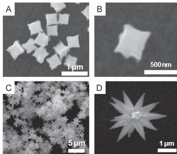
**Fig. 3.** A and C are the large area SEM images of mesostructures obtained from 1,2-PDA and aniline respectively by increasing their precursor monomer concentration three times from that of their optimum concentration. B and D are corresponding single images.
