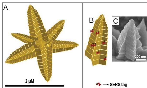
**Fig. 10.** Schematic representation of the mesoflower showing its unique morphology. Models of a single mesoflower (A) and a single stem (B). (C) Enlarged SEM image of a single stem of the mesoflower.
