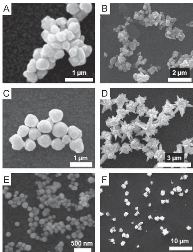
**Fig. 7.** SEM images of the various precursor-coated gold nanoparticles after growth (A)  $\beta$ -naphthyl amine; (B) thiophene; (C) pyrrol; (D) 1,4-PDA; (E) 1,4-aminophenol and (F) p-nitroaniline. The concentration of the precursors used during the seed preparation was 0.2 M.
