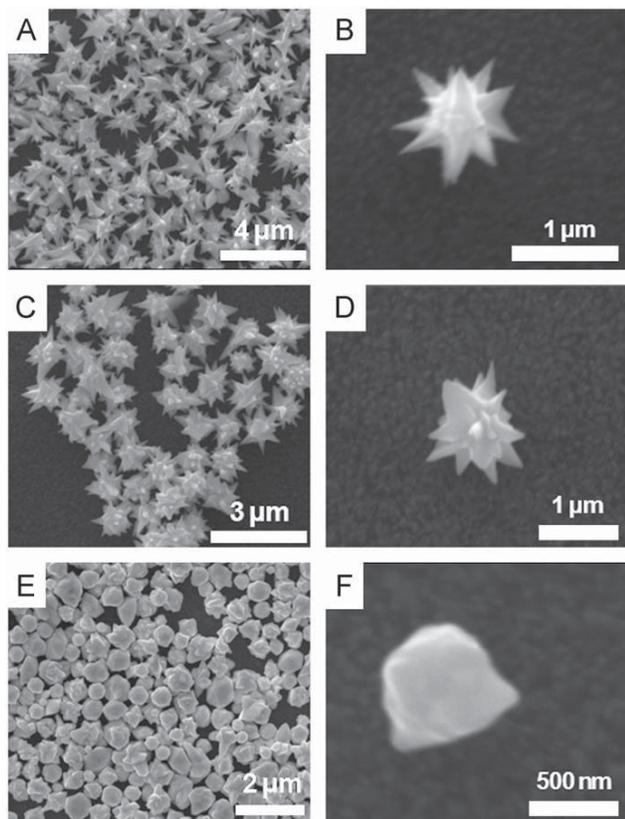
**Fig. 2.** A, C, and E are the SEM images meso/nanoparticles formed when the reaction carried out using seed nanoparticles synthesized by varying concentrations of 1,2-PDA. (A) 0.1 M; (C) 0.02 M and (E) 2 mM. B, D, and F are the corresponding single images of A, C, and E, respectively.
