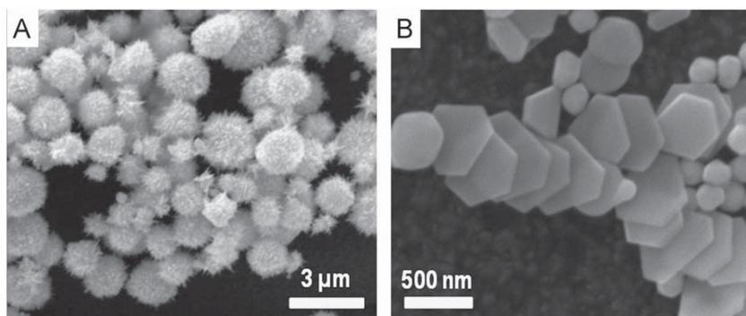
**Fig. 6.** (A) SEM image of meatball-like mesostructures formed when the growth carried at room temperature by keeping all other parameters constant. (B) Nanoplates formed when the reaction was conducted in the absence of  $\text{AgNO}_3$ .
