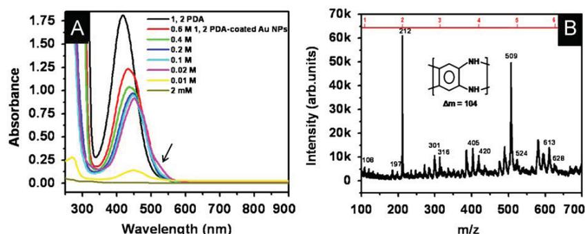
**Fig. 5.** (A) UV–vis absorption spectra of 1,2-PDA and oligo-1,2-PDA-coated gold seed nanoparticles prepared by varying the concentration of 1,2-PDA added during preparation of the seed. (B) LDI mass spectrum of the oligo-1,2-PDA-coated Au nanoparticles seeds. Fragmentation peaks of oligo-1,2-PDA are marked in the spectrum.
