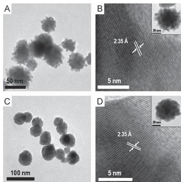
**Fig. 8.** TEM images of the oligo-1,2-PDA-coated Au nanoparticles (seeds) prepared by using (A) 0.2 M 1,2-PDA during seed preparation which leads to mesoflowers after growth; (B) its lattice resolved image; (C) large area image of seeds prepared by using 2 mM 1,2-PDA during seed preparation which leads to quasispherical particles after growth and (D) its lattice resolved image. Insets in B and D are corresponding single particles.
