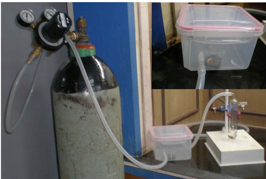
Figure S1. Photograph of the set-up used for the formation of Au@SGAN and Au@MSA SLs. Inset shows a magnified view of the plastic vessel used for the SL formation. The grown SL film is seen faintly.
