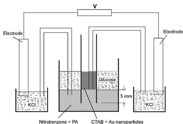
Fig. 1. Schematic of the experimental setup used for studying potential oscillations. 5 mm of the 2 cm diameter tube is dipped into the organic solution and the dipped end of the tube is given a notch of 1 mm. The cell is completed using two salt bridges and Ag/Ag<sup>+</sup> electrodes. The monolayer is formed at the CTAB–nitrobenzene interface.
