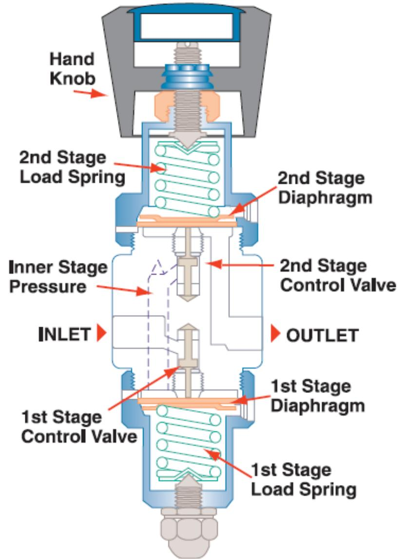
Regulators are equipped with CGA (Compressed Gas Association) fittings for connection to cylinders. Each CGA connection has a numerical designation, and a listing of gases with which it may be used.
